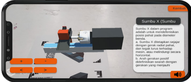
c) X-axis point simulation of CNC lathe training unit-2A
